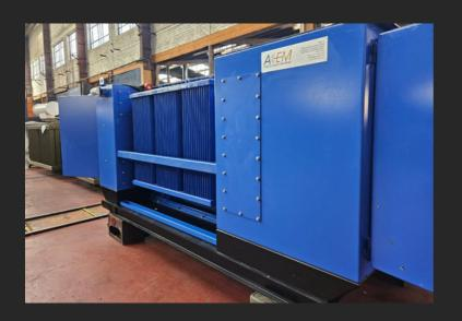
The 630kVA 11000/1000V 3Ph 50Hz Medium Voltage Underground Miniature Substation stands as a pioneering solution for the robust and safe operation of electrical equipment in the demanding underground mining environment. Equipped with cutting-edge safety features such as the Neutral Earthing Resistor Professional Monitoring Panel (NERPRO) and the Battery Trip Unit (BTU), this system exemplifies the utmost commitment to human safety and the protection of critical equipment.
