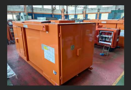
The project involved the design, manufacture and testing of an ANAF (Dry Type) Medium Voltage skid-Substations for the Jwaneng Mine a critical component of the mines early works extension. The end user, a leading entity in Botswana's mining sector, required customized, durable Dry Type Medium Voltage Skid Substations (MVS) to meet the harsh conditions of the mine. The project focused on ensuring the substations' resilience, safety, and operational reliability in the surface mining industry.
